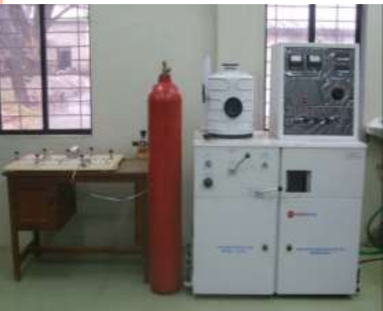
P C Isotherm: For H 2 storage behavior of material
