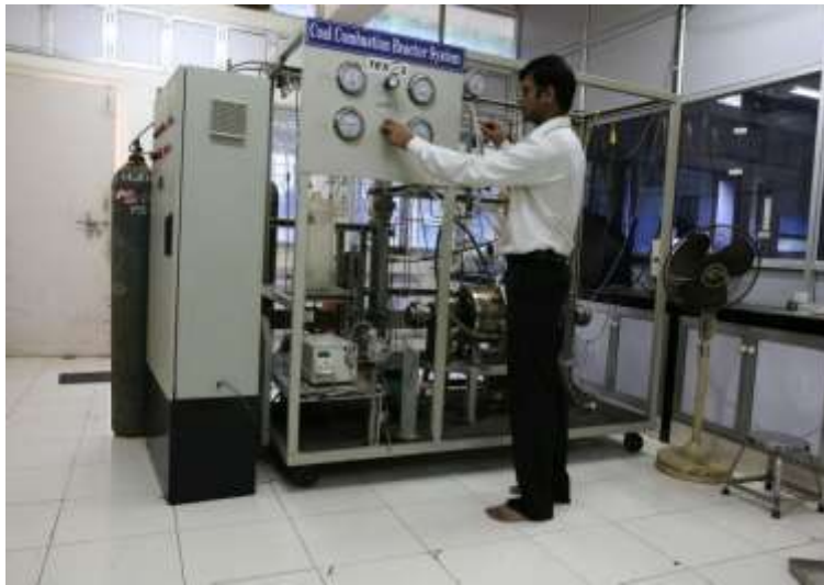
Fixed Bed Reactor for Study of Underground Coal Gasification
