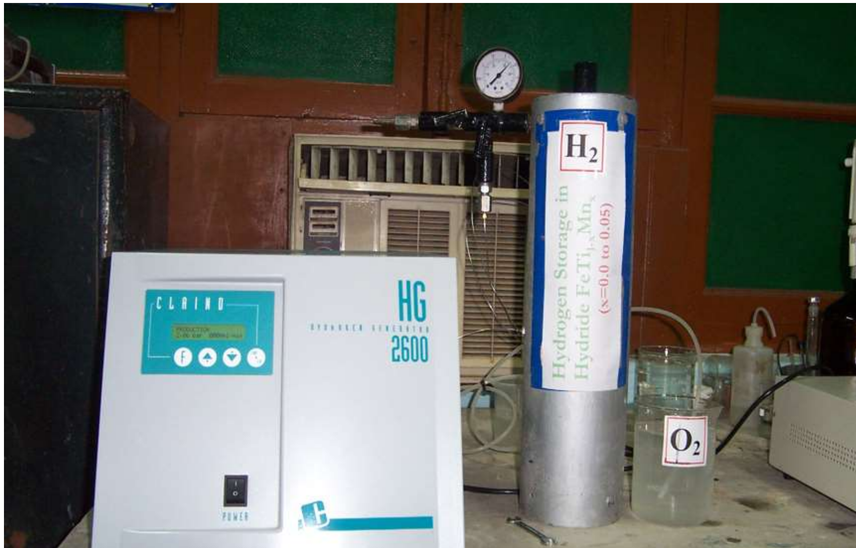
Hydrogen produced by PV driven electrolysis stored in hydride tank
